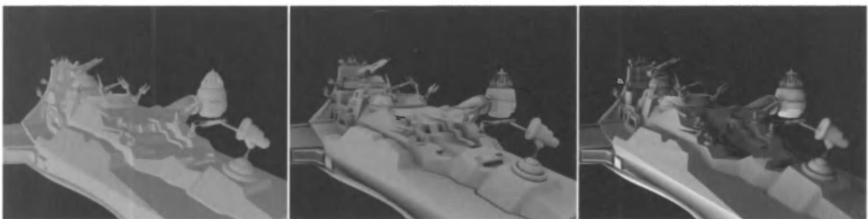
Figure 9.72. Three renderings of a model from the game Warhawk by Incognito Entertainment. The model uses a gray Lambertian material in all three renderings. On the left, the model is rendered with direct lighting and no shadowing. In the center, it is rendered with ambient light and ambient occlusion. On the right, it is rendered with precomputed radiance transfer, with a strong light from the left. (Images courtesy of Manchor Ko.)
