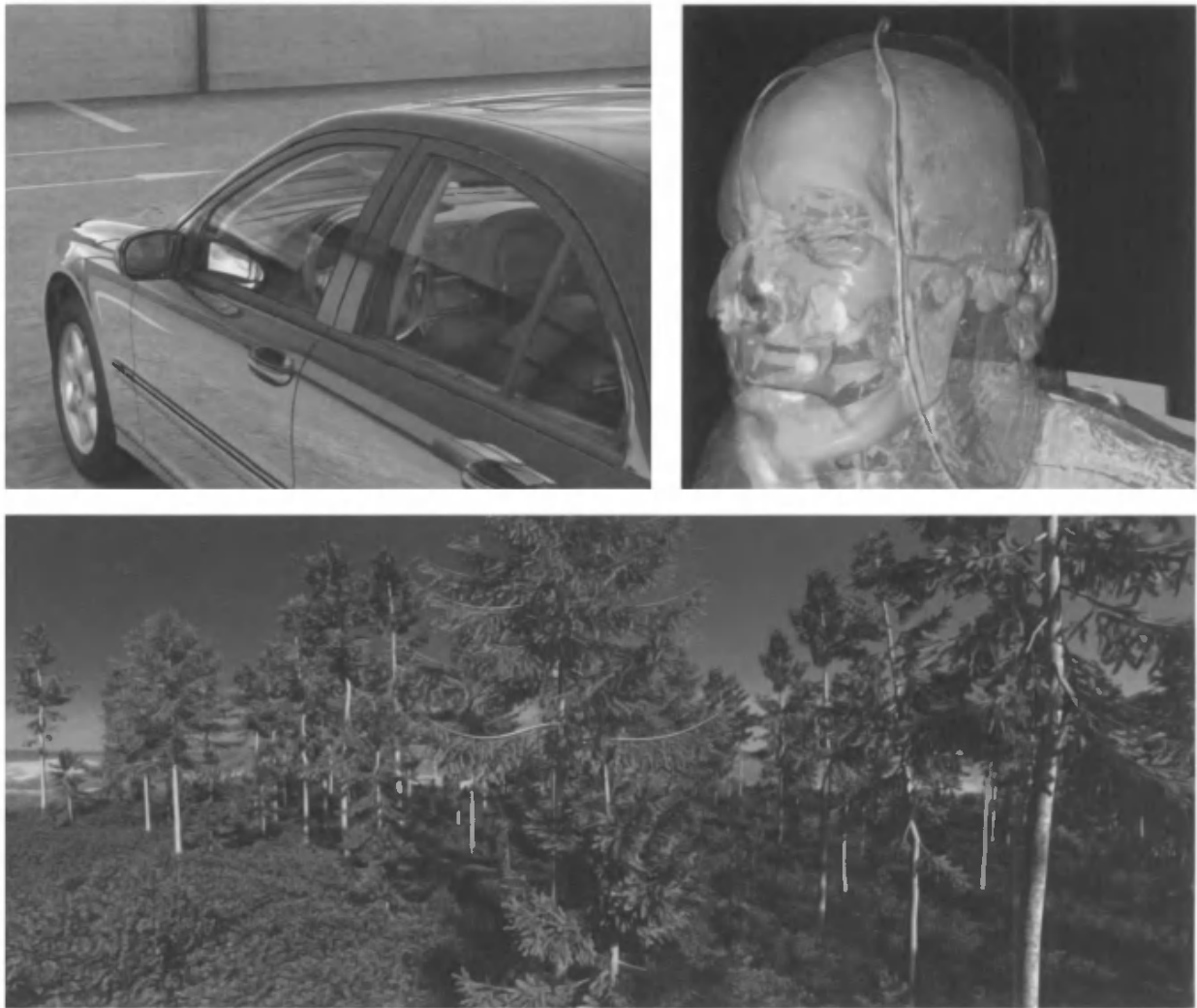
Figure 9.62. Three areas where interactive ray tracing can excel. In the upper left image, true reflections and refractions are computed. The free-form surfaces from the model are directly ray traced without having to convert them into triangle meshes, allowing physically precise visualization. In the upper right, volumes are visualized directly via rays, without the need to explicitly find the surfaces before rendering. The lower image shows a scene with 1.5 billion potentially visible triangles. It is very costly because of the many alpha textured leaves. On 16 Opteron cores using untuned code (no SSE) it runs at about 2 fps (one directional light, 640x480). ( Images courtesy of Computer Graphics Group, Saarland University. )
