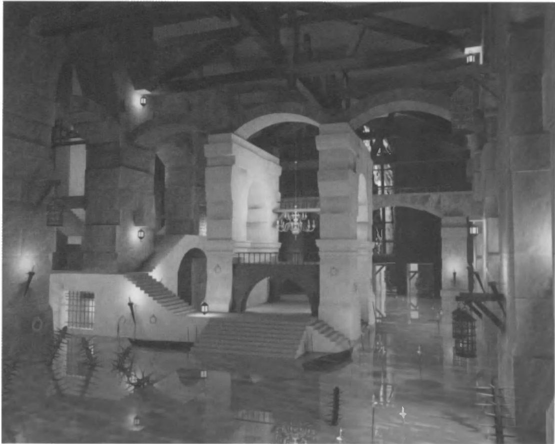
Figure 9.42. The water reflection is performed by mirroring polygons through the water's surface and blending them with the textured water polygon. The chandelier and some other elements are replaced with sets of textured polygons. ( Image courtesy of Agata and Andrzej Wojaczek [agand@aga3d.com], Advanced Graphics Applications Inc. )
