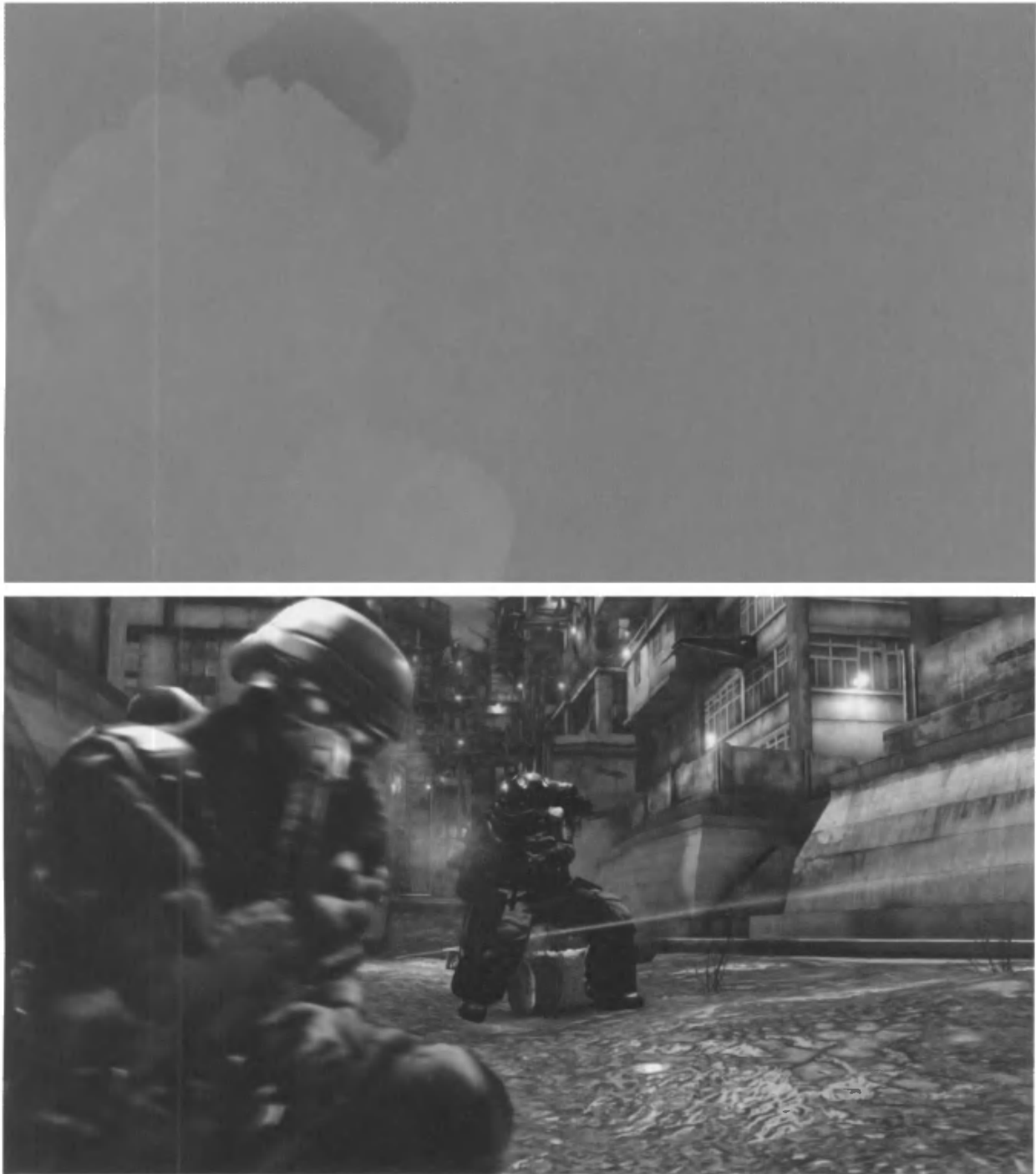
Figure 10.34. The top image is a visualization of the velocity buffer, showing the screen-space speed of each object at each pixel, using the red and green channels. The bottom image shows the effect of blurring using the buffer's results. ( Images from "Killzone 2," courtesy of Guerrilla BV. )
