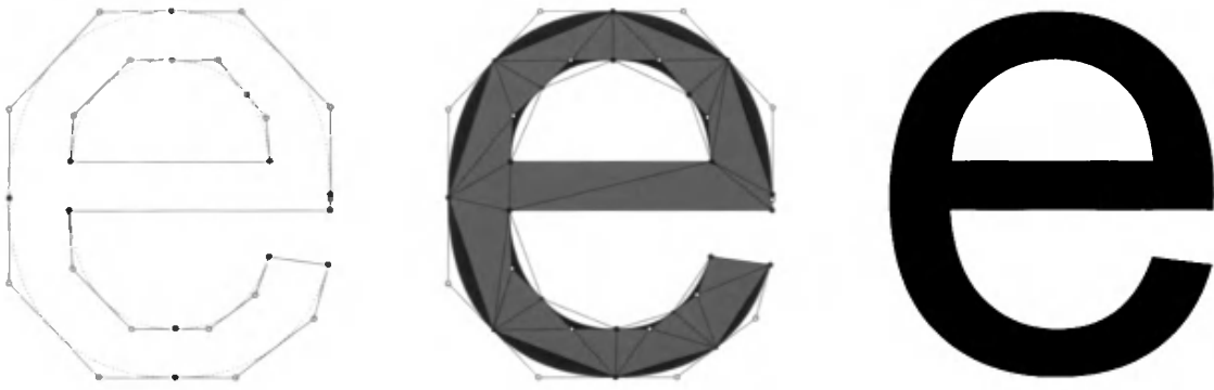
Figure 13.8. An e is represented by a number of straight lines and quadratic Bézier curves (left). In the middle, this representation has been “tessellated” into a number of bounded Bézier curves (red and blue), and triangles (green). The final letter is shown to the right. ( Reprinted with permission from Microsoft Corporation. )
