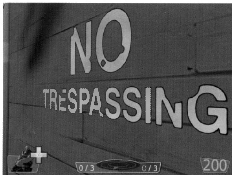
Figure 6.11. A vector texture used to display crisp text. The original “no trespassing” sign’s data is held in a 64 \times 64 distance field. The outline around the text is added by mapping a particular distance range to the outline color [439]. (Image from “Team Fortress 2” courtesy of Valve Corp.)
