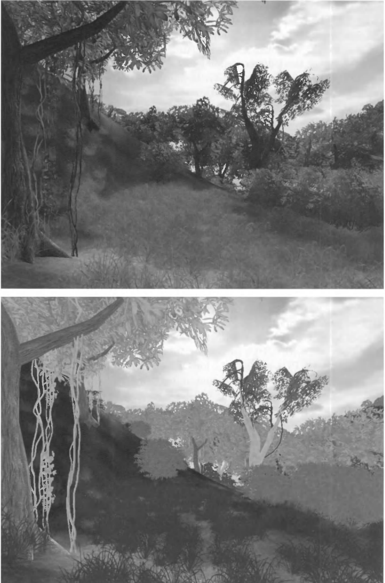
Figure 15.3. Vegetation instancing. All objects the same color in the lower image are rendered in a single draw call [1340]. ( Image from CryEngine1 courtesy of Crytek. )
