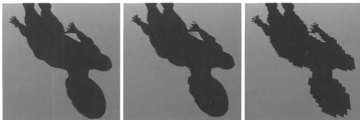
Figure 9.23. On the left, a 2048 \times 2048 shadow map rendering of a shadow. In the middle, a 256 \times 256 shadow silhouette map provides a considerably better shadow than the 256 \times 256 standard shadow map on the right. (Images courtesy of John Isidoro, ATI Research, Inc.)
